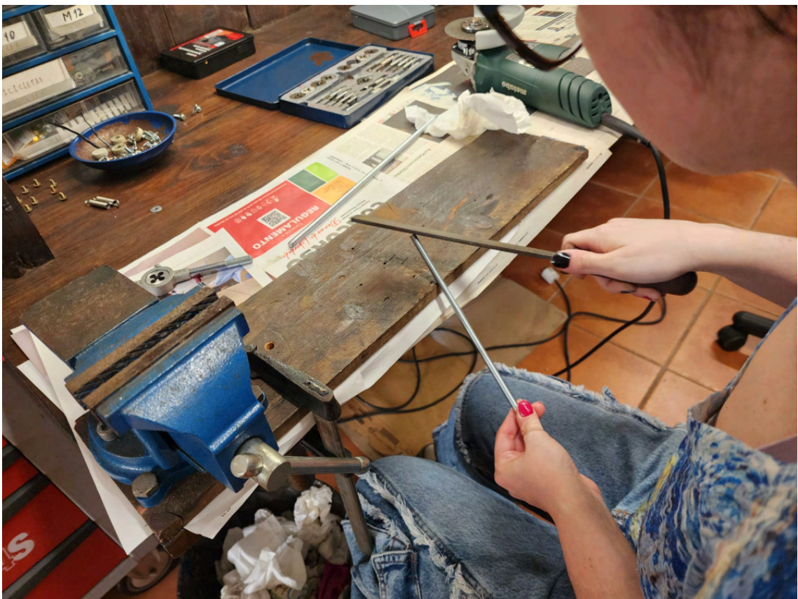
Figure 6.15: Metal Rod trimming process
