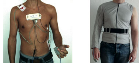
Fig. 13. Left: SENSATRON system attached to a subject by standard adhesive electrodes. Right: functional textile as user-interface developed within HeartCycle for the SENSATRON device.
