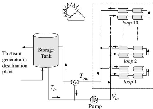
Fig. 3. Distributed solar collector field schematics.
