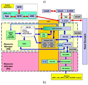
Fig.2. The EuQoS model; a) The high level EuQoS architecture; b) The main building blocks.
