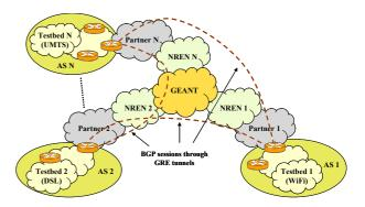
Fig. 1. Access networks, NRENs and GEANT architecture.
