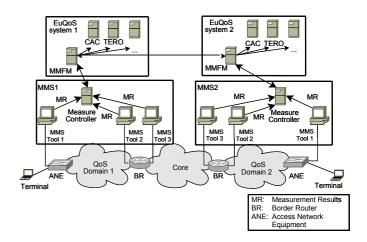
Fig.5. The Monitoring and Measurement System (MMS).
