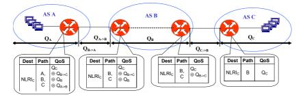
Fig.6. Example of EQ-BGP operation.
