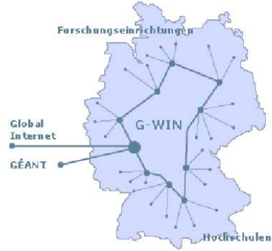
Fig. 3. Representative two layer (Tier-I and II) ISP topology of the German Research Network (DFN - G-WIN). Large points belong to the Tier-I (core) layer, small points are Tier-II layer access routers.
