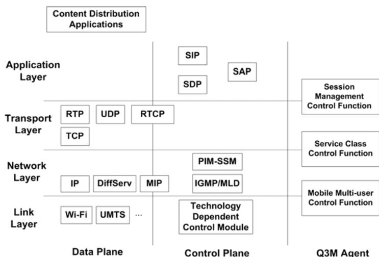
**Figure 4 - Q3MA: control functions integrated in the TCP/IP protocol stack**
