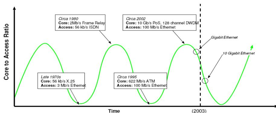
**Figure 1 - Relative core to access bandwidth ratio over time [7]**
