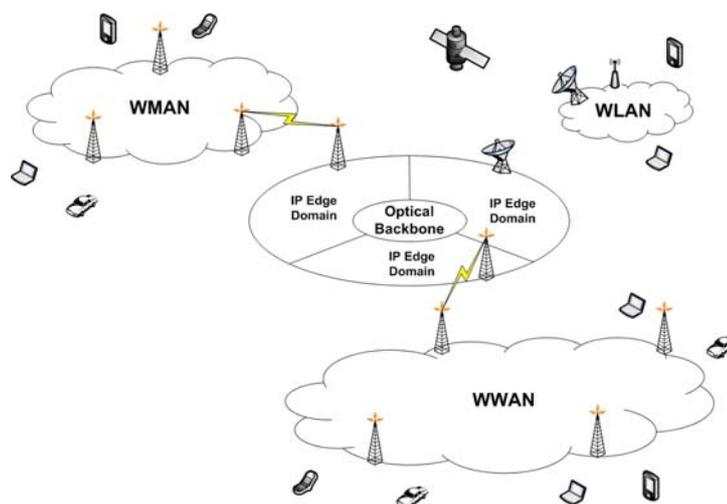
**Figure 2 - Heterogeneous IP network infrastructure**
