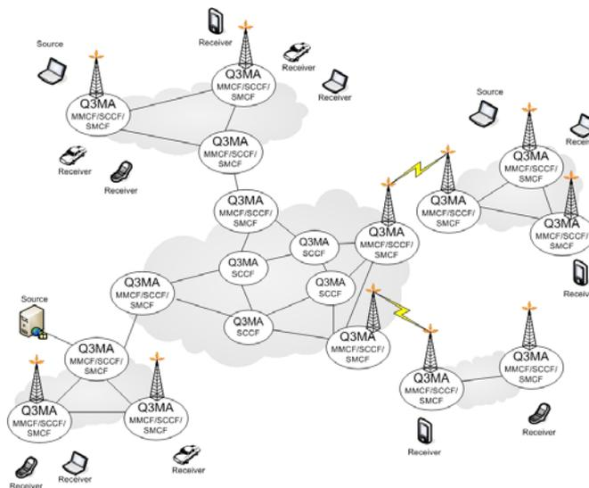
**Figure 3 – Location of the Q3M control functions in a general scenario**
