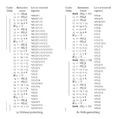
Figure 21.5: Execution of a dot-product loop, with 4-word cache blocks.
