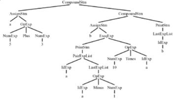
Figure 1.4: Tree representation of a straight-line program.
