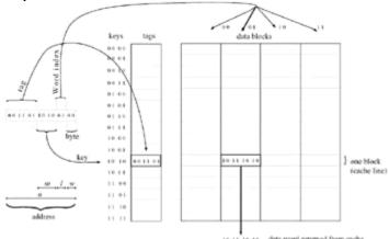
Figure 21.1: Organization of a direct-mapped cache. *Key* field of the address is used to index the *tags* array and the *data blocks*; if tags[*key*] matches the tag field of the address then the data is valid (cache hit). *Word index* is used to select a word from the cache block.
