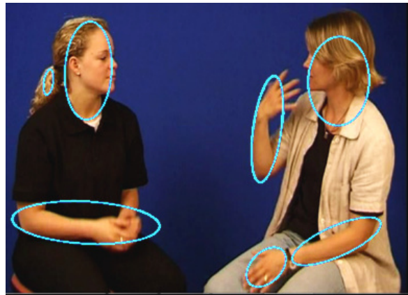
Figure 3. This figure shows the results of body part tracking, based on a previous skin-color detection step, for one frame. Note that no explicit body model is used by this detector at the moment.
